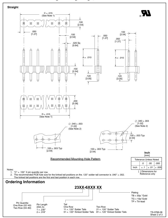
$3M^{™}$  Pak 100 Pin Strip Header .100" and .100" × .100" Straight and Right Angle, Solder Tail
