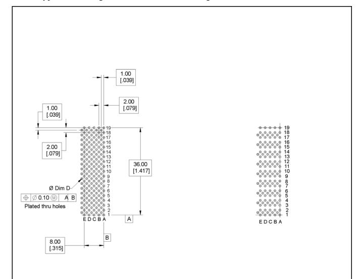
Recommended PCB hole mounting pattern for coaxial, column differential and stripline applications
