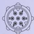
7-position B-key #26 Pin Contact
