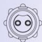
2-position #20 Socket Contact
