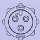
3-position #20 Pin Contact
