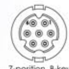
7-position B-key #26 Socket Contact
