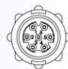
7-position B-key #26 Socket Contact
