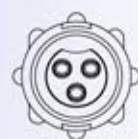
3-position #20 Socket Contact
