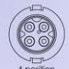
4-position #22 Pin Contact
