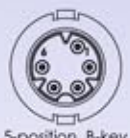
5-position B-key #26 Pin Contact
