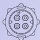
4-position #22 Pin Contact
