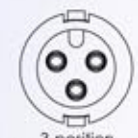
3-position #20 Socket Contact
