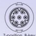
7-position B-key #26 Pin Contact
