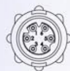
6-position A-key #26 Socket Contact
