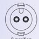
2-position #20 Socket Contact
