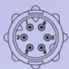
6-position A-key #26 Pin Contact
