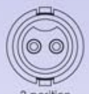
2-position #20 Pin Contact
