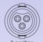
3-position #20 Pin Contact
