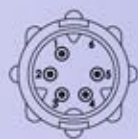
5-position B-key #26 Pin Contact
