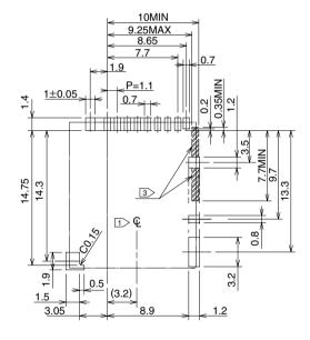
Note 1 6 indicates the center line of the microSD card slot.
