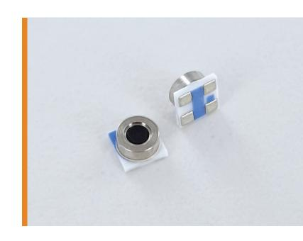
This MEMS based sensor includes a high-linearity pressure sensor with ultra-low power 24-bit digital output ( $I^2C$ ) and an altitude resolution at sea level of 13 cm. The board level design delivers sensing accuracy for both pressure ( $\pm 0.5$  mbar) and temperature ( $\pm 2^{\circ}C$ ) measurements.
