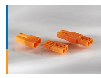
TE Connectivity (TE)'s 2 position wire-to-wire connector provides a space-saving solution for indoor downlighting, connecting power to luminaire. Designed with limited space in mind, the low profile, UL/CSA 2459 compliant connector eliminates the hazard of electric shock and accepts 18 AWG – 22 AWG solid or tin-dipped stranded wires. It is designed for easy, tool-free installation and eliminates mis-mating through its bump feature.
